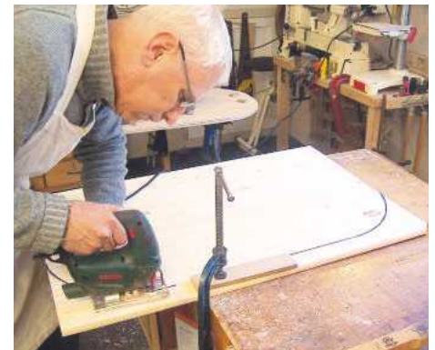
▲ Pic.4 A jigsaw makes short work of cutting the overall shape
